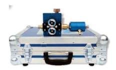
BDJ BUDGET micro cable blowing machine is dedicated for last miles of FTTH network. Depending on the quality of the laid micro duct route and cable stiffness, BDJ Budget can be used to blow cable sections up to 700m. The machine is very easy to use. BDJ BUDGET is powered by a cordless screwdriver. By using the overload clutch of the screwdriver, the desired power of the roller drive, can be set very precisely.
