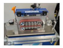
BDJ Standard is a professional blowing machine designed for blowing micro cables. A solid and simple construction ensures easy operation and a longevity of the unit. Machine is equipped with a high quality belt feeder and pneumatic motors. Basic version has a mechanical counter meter pre-installed. Upon request we provide electronic counter with a speed measurement function.
